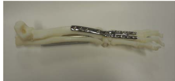
Fig. 5. Tailor-made metal bone plate (COBARION)
