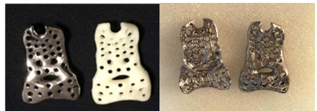
Fig. 8. Examples of tailor-made metal bone plates(COBARION, ABS resin, and T-ALLOY TOUGH(back, front side))
