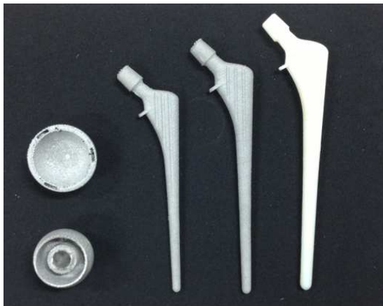
Figure 5 Stem, cap, socket constructed by an EBM device
