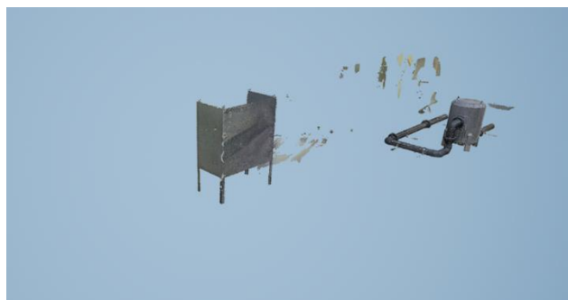
Fig. 4 t_0 - t_1 Differential extraction (error threshold 0.2 m)
