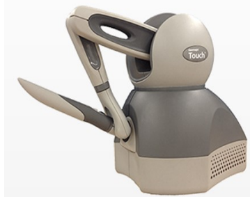
Fig.3. Tactile device with force feedback used in APT (Geomagic Touch)
