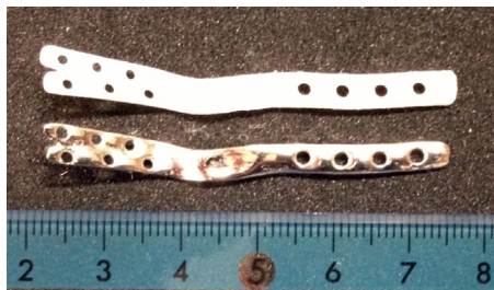
Fig. 28. Manufactured plates for affixing to the fractured bones of the respective dogs.
