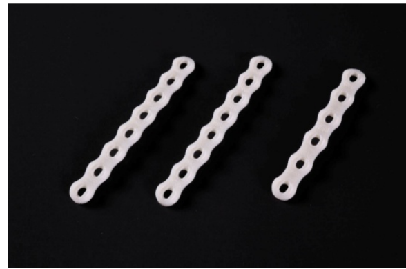
Fig. 23. Several tailor-made plate models manufactured with a 3D printer.
