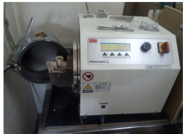
Fig. 25. Vacuum-pressure casting machine.
