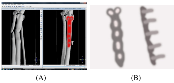
Fig. 2. (A) Example of a sketch prepared by a veterinarian using the proposed design system. (B) Front and side views of a manufactured plate.
