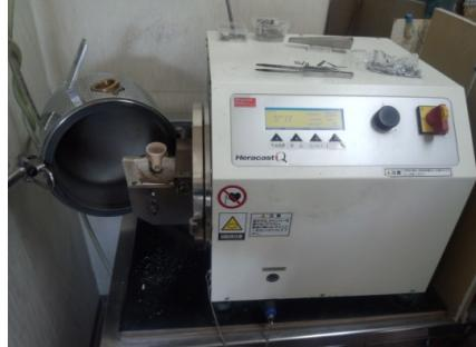
Fig. 12 Vacuum-pressure casting machine
