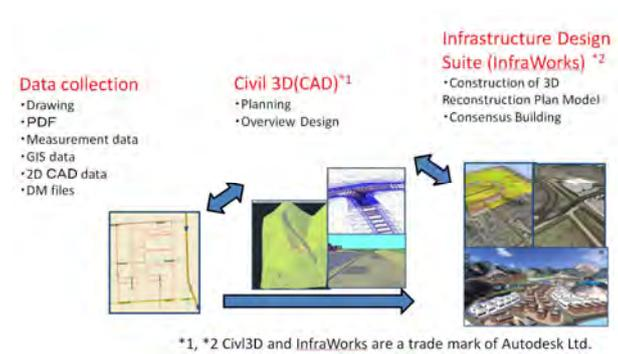
Fig. 1. Workflow for building a 3D map
