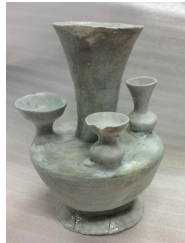
Fig. 10 Replica fabricated using the ZPrinter 250
